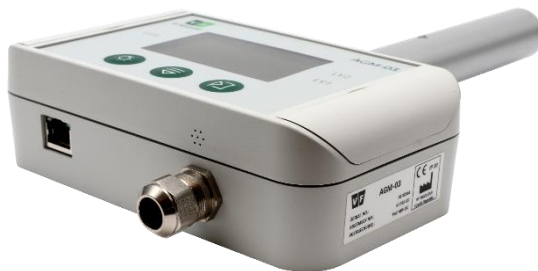
AGM-03 with an optional RS-485 interface and relay outputs
