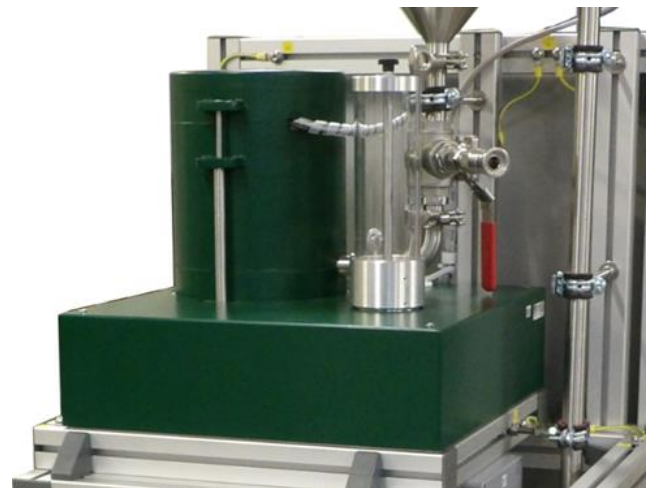
Detail of the detector and the container with unused iodine cartridges
