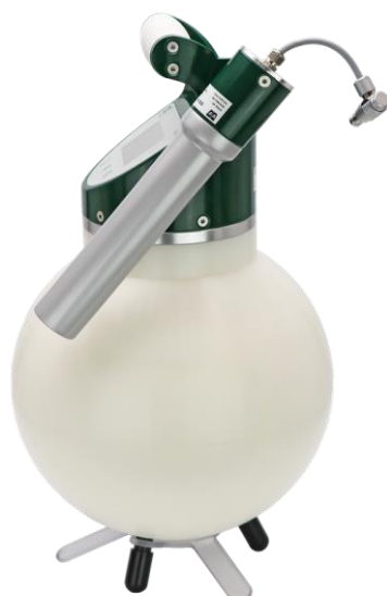
PNM-02 with SGD-01e probe for the measurement of gamma dose equivalent rate (transport position)
