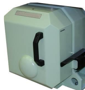
Shielded sampling chamber with filters and dose rate meters
